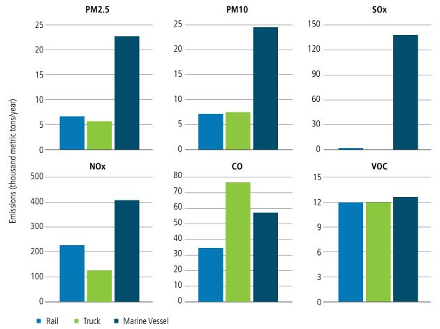
Figure 7-4. Air Emissions from the Transportation of Coal and Liquid Fuels, by Transport Mode<sup>80, s</sup>
