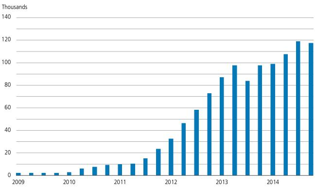
The rapid increase in crude by rail is a function of the growth in new source of new oil production, particularly in North Dakota, as well as limited pipeline capacity for moving this oil to refiners on the East and West Coasts.
