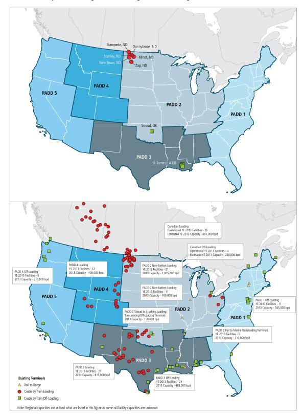
Figure 5-2. Crude Oil by Train Loading, and Offloading, and Rail-to-Barge Facilities for 2010 and 2013<sup>17</sup>
