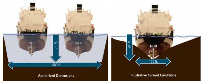
Figure 5-9. Calcasieu River Ship Channel, Illustration (not to scale) of Authorized Dimensions and Example Conditions Where Shoaling Occurs<sup>78</sup>
